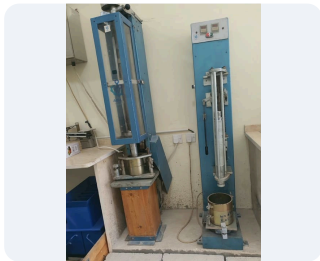
Automatic compactors: Proctor and Marshall
