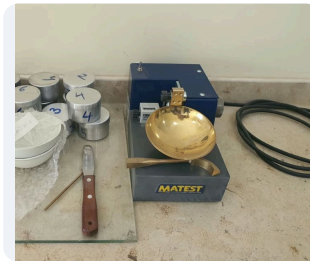
Casagrande liquid limit device
