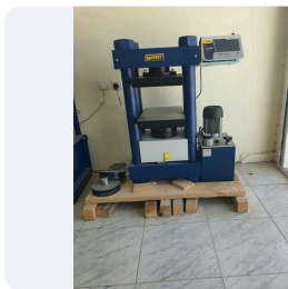
Digital compression testing machine
