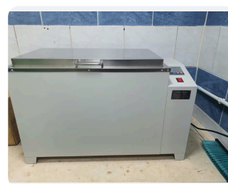
Water bath for Marshall specimens
