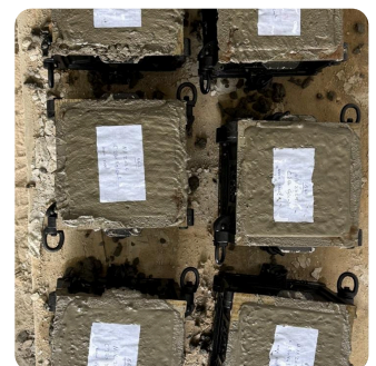
Casting concrete cubes on site
