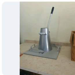
Slump cone and tamping rod
