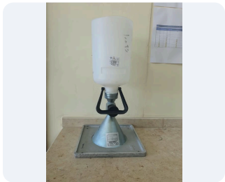
Sand-cone apparatus — field density
