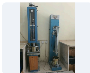
Automatic compactors: Marshall and Proctor
